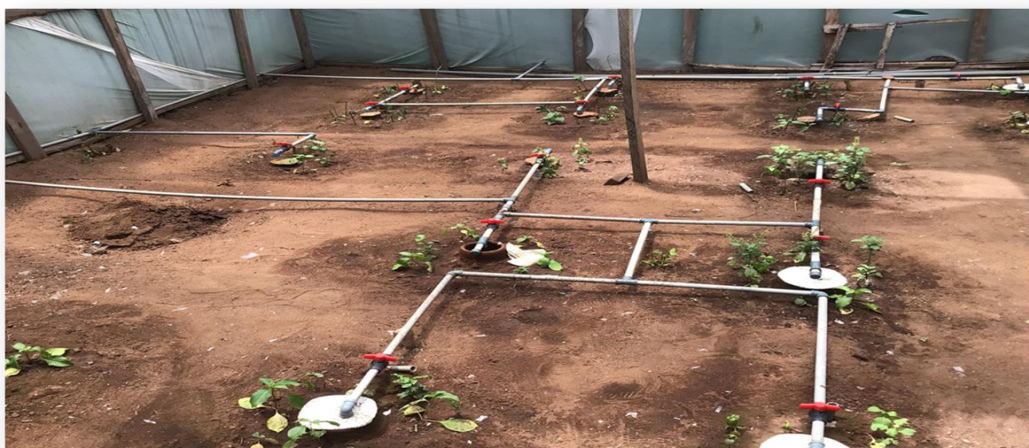
Plate 1: Porous Clay Pot Experimental Set up
