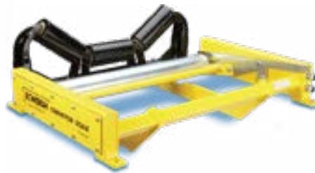
Tecweigh's WY10 legacy belt scales feature single and dual idler versions ideal for installation on primary belts where high impact and shock force loading applications are encountered. A self-storing calibration weight makes routine checks easy and safe. Plus, the weight can always be found mounted in the belt scale frame.
