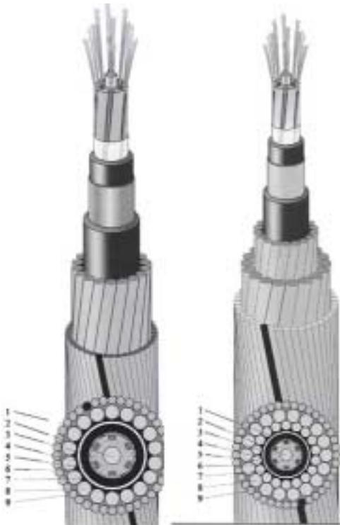
Figure 2: 15-t SA and 40-t DAH armoured cable
