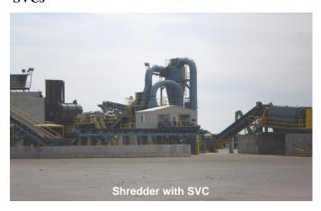
SVCs (static VAR compensators) are a proven way to meet utility flicker requirements. These systems are installed on the main power feed to the motor, or where the operation interfaces with the power company. With a properly-designed SVC, an operator can meet utility requirements, and simply run their business.
